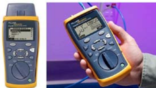
Rys. 4.4. CableIQ Qualification Tester firmy Fluke Networks [4].
