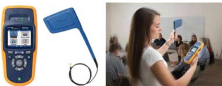
Rys. 4.8. AirCheck Wi-Fi tester firmy Fluke Networks [4].
